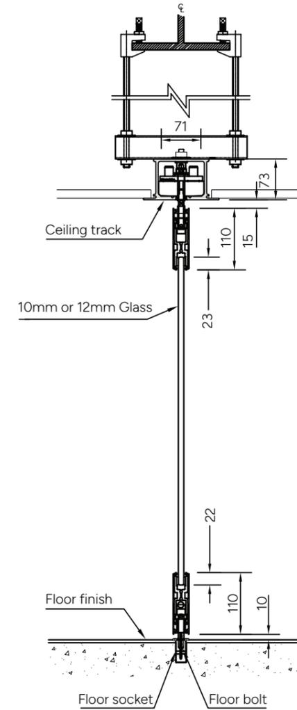
**Vertical Section of Panel & Track Fixing**
